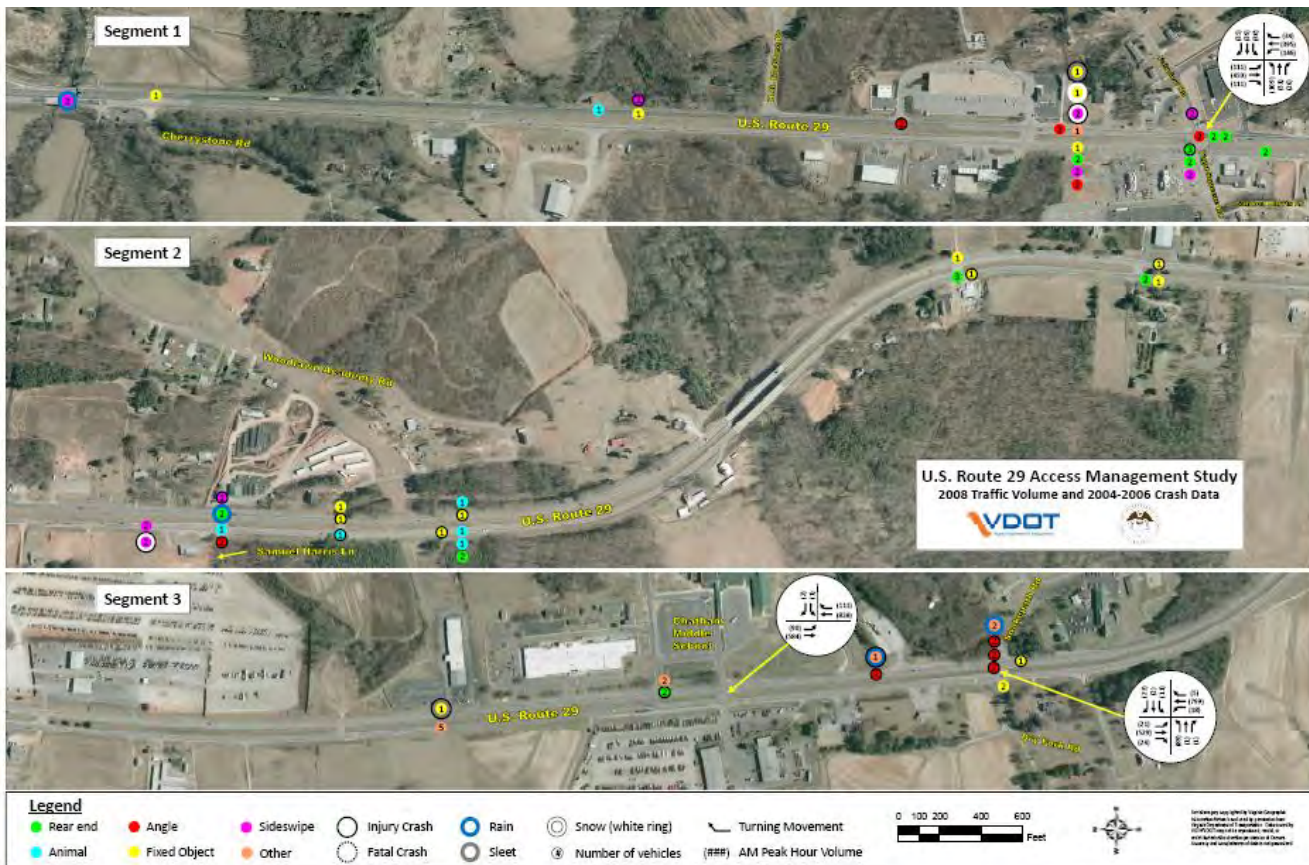
Figure 2.3: Crash data inclusive of 2004 – 2006, and 2008 turning movements along the Seminole Corridor - U.S. 29 south of Chatham, U.S. Route 29 Access Management Study.
