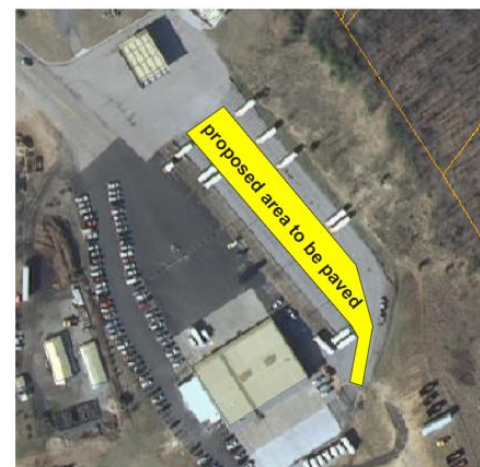
Figure 5-2: School Bus Parking Lot Access Lane
